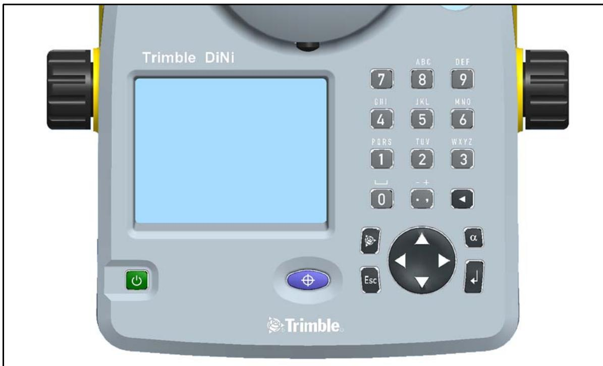
Figure 3.6 Control and display unit of DiNi®
